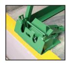
The installer adjusts the leveling bolts on the front and rear supports using a standard  $\frac{1}{2}$  square head socket.
