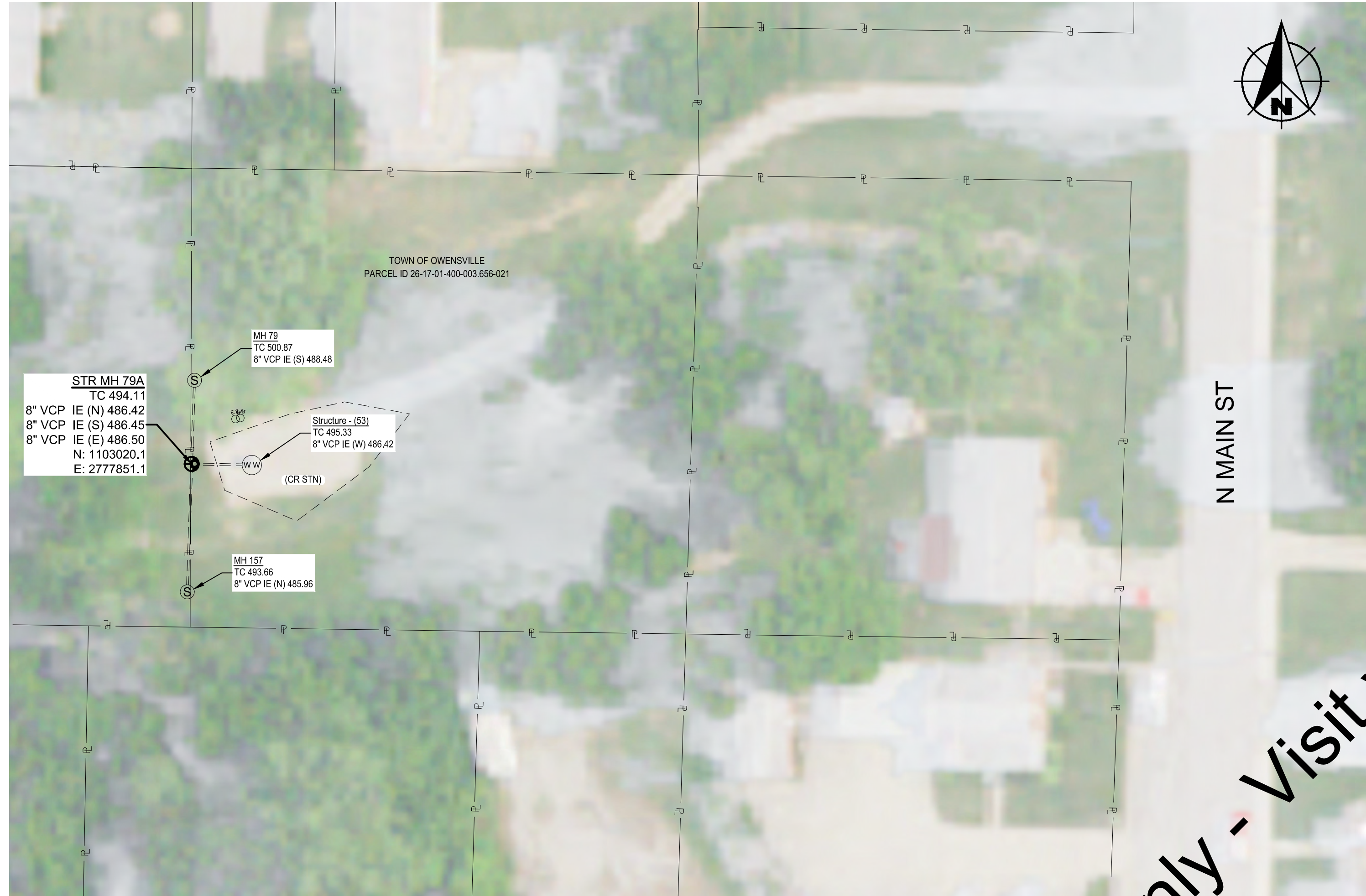
PLAN - NEW MANHOLE INSTALL AT HILLCREST LIFT STATION SCALE: 1" = 30'
