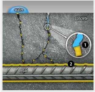
1. Hydrophobic pore blocking
